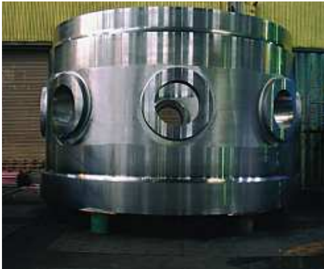
Reactor pressure vessel monobloc upper shell for the Olkiluoto 3 (Finland) EPR™ reactor pressure vessel.
