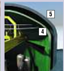
The reactor containment building has two walls: an inner pre-stressed concrete housing (4) internally covered with a metallic liner and an outer reinforced concrete shell (5).
