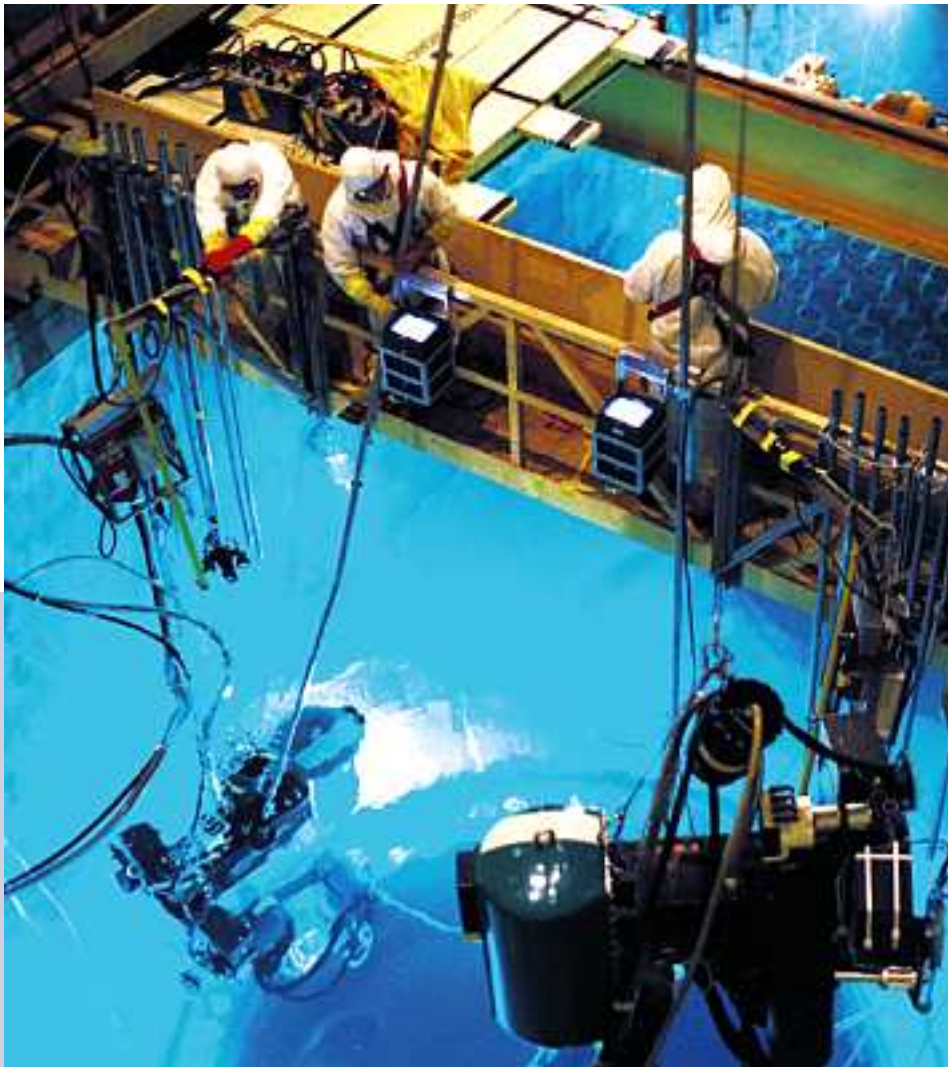
In-service inspection machine for ultrasonic testing of reactor pressure vessels.
