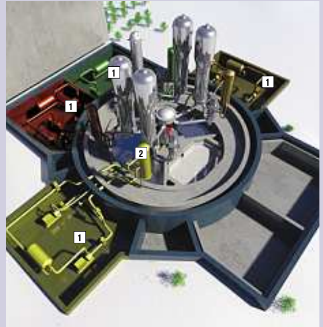
The major safety systems comprise four sub-systems or trains, each capable of performing the entire safety function on its own. There is one train in each of the four safeguard buildings (1) surrounding the reactor building (2) to prevent a simultaneous failure of the trains.
